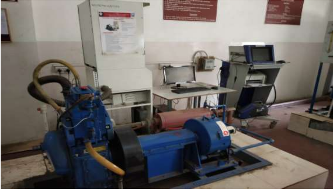
Figure No. 2.7: Diesel Engine Setup
